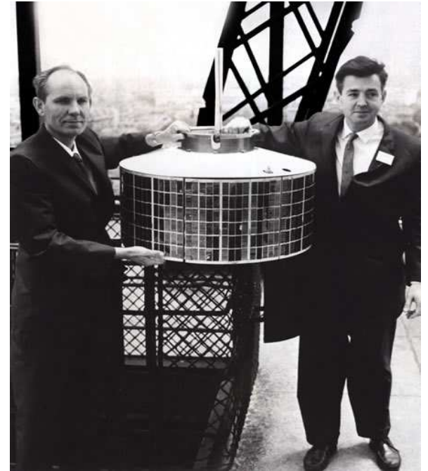
Syncom 3: 8/64 GEO Comsat 68 kg w. propellant
