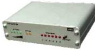
Figure 1 The front panel of the R2FX showing the various LEDs
